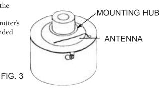
5. Secure the receiver housing to the mounting hub by sliding the housing onto the 3 screws on the hub and turning clockwise. Tighten the 3 screws when in place.
